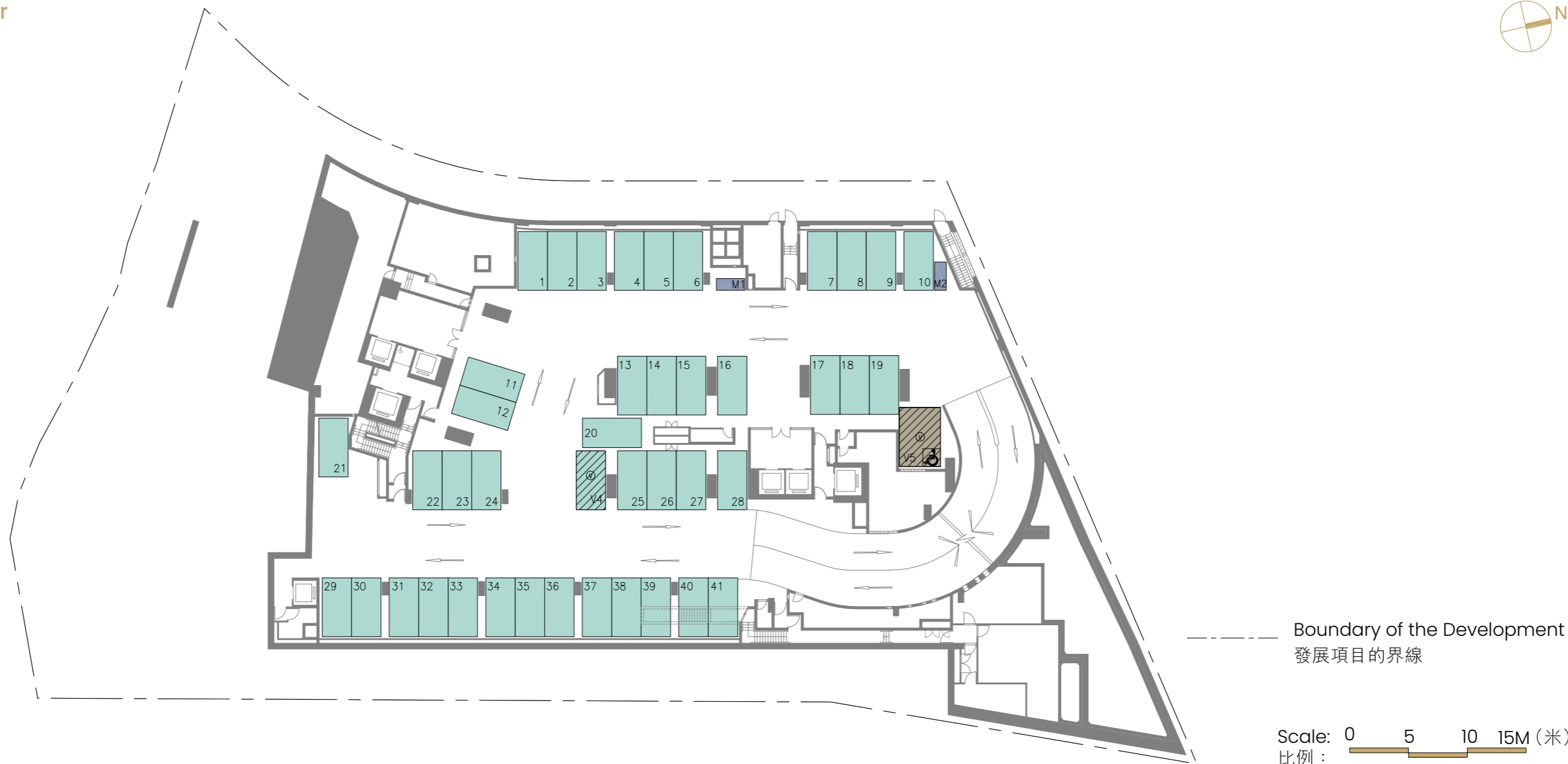
Location, Numbers, Dimensions and Area of Parking Spaces 停車位位置、數目、尺寸及車位面積
